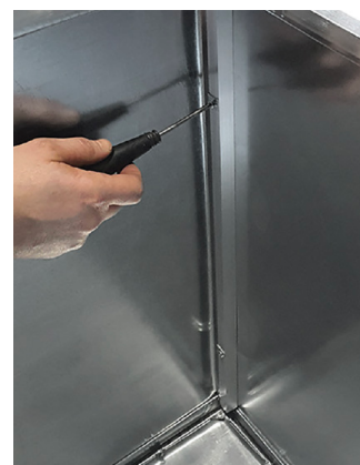
Screw the side parts with screws B.
